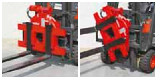
CONTENITORI RIBALTABILI CON CARRELLO ELEVATORE A FORCHE ROTANTI DUMPING CONTAINERS WITH ROTATING FORKLIFT TRUCK
